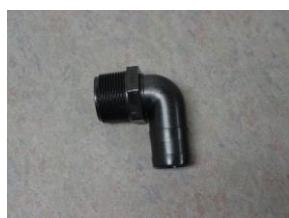
**C - Overflow Installation:** Thread in the overflow elbow into the 1½" hole near the top of the barrel. This is a tight fit, so it will require some elbow grease to get the threads started. You may need to use a file to open up the hole a little bit. Thread this all the way in, and stop when the barbed side of the elbow is pointing toward the ground, slip a five foot section of the sump drain kit hose onto the elbow.
