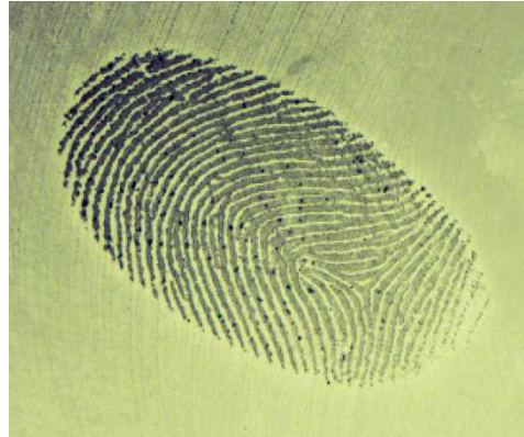
Figures 3 & 4. Metal Unedited Print & Metal Edited Print, respectively. 6% concentration, 75% relative humidity, 10 minute saturation time, 120°C, 20 minute fume time.
