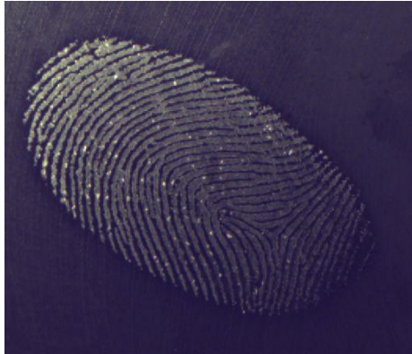
Figures 3 & 4. Metal Unedited Print & Metal Edited Print, respectively. 6% concentration, 75% relative humidity, 10 minute saturation time, 120°C, 20 minute fume time.
