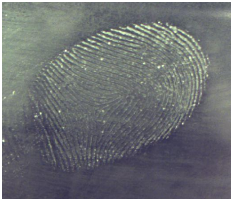
Figures 3 & 4. Metal Unedited Print & Metal Edited Print, respectively. 6% concentration, 75% relative humidity, 10 minute saturation time, 120°C, 20 minute fume time.
