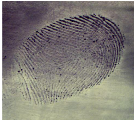
Figures 3 & 4. Metal Unedited Print & Metal Edited Print, respectively. 6% concentration, 75% relative humidity, 10 minute saturation time, 120°C, 20 minute fume time.
